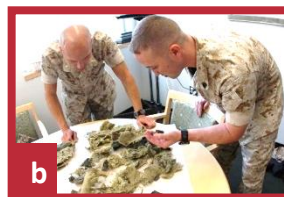
b. Pieces of a Kevlar helmet used to help absorb the blast of a grenade
