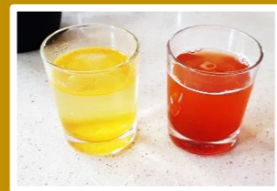
Yellow in acidic solution and red in alkaline solution
