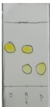
Figure 3: An example of TLC of o- and p-nitroaniline along with their mixture has shown here.
